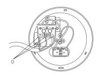
4. Connect the eletrical cable with terminal strip (D).
