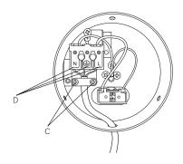
Unscrew the two screws (C) from the back of the lamp housing. Press N, ⊕, L tabs on terminal strip (D) to pull the cable out.
