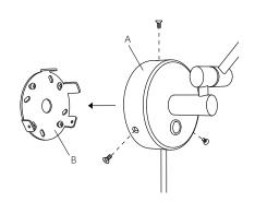
3. Attach the lamp body (A) back to the wall mounting (B).
