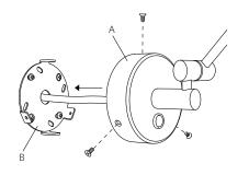
5. Attach the lamp body (A) back to the wall mounting (B).
