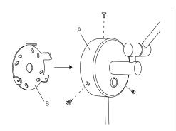
1. Remove the wall mounting (B) by unscrewing three screws from the lamp body (A).
